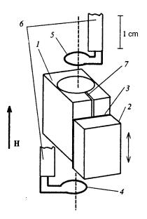
FIG. 2. Block diagram of the resonance circuit: (1) cavity; (2) movable copper plate; (3) thin insulating film; (4, 5) coupling loops; (6) coaxial leads; (7) narrow slot.
